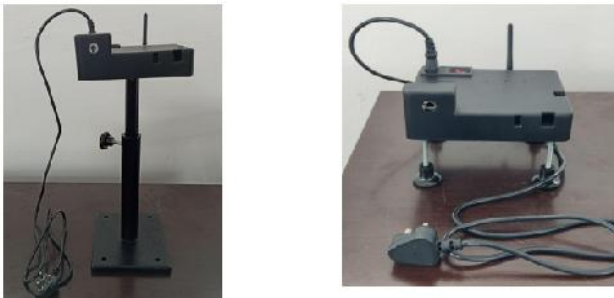
Fig. 5&6. Sensor Node for Broiler and Layer farms
